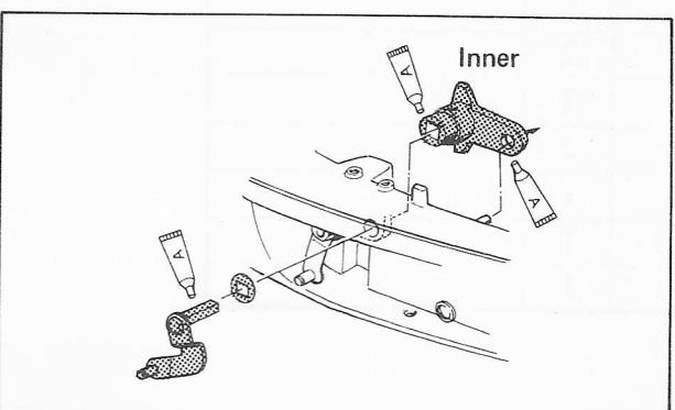
5. Apply grease to the shift control lever (inner) and install it to the bottom cowling and the link rod.
