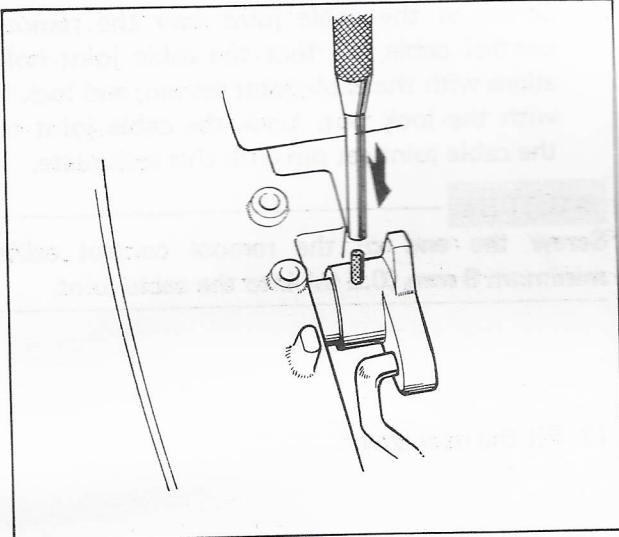
7. Align the spring pin holes and drive the spring pin into the hole by using rod driver and a hammer.
