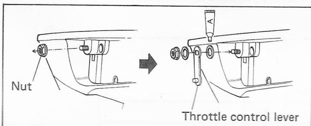
3. Remove the nut from the throttle control lever shaft and re-install parts with the throttle control lever as shown in illustration.
