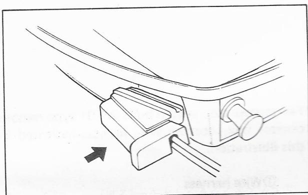
8. Install the rubber grommet to the bottom cowling. Lead the wire harness through the grommet if it is necessary.
