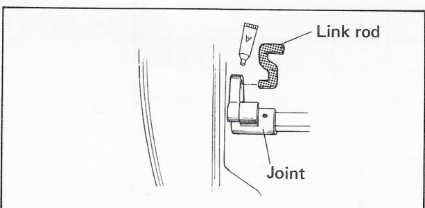
4. Insert the link rod into the joint hole and hold it vertically.
