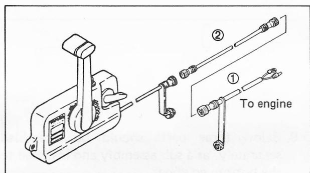
For remote stop switch built in 701 type remote control box, use the wire harness indicated in this illustration.
