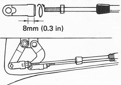
11. Screw in the cable joint over the remote control cable, so that the cable joint hole aligns with the cable joint set pin, and lock it with the lock nut. Lock the cable joint to the cable joint set pin with this lock plate.
