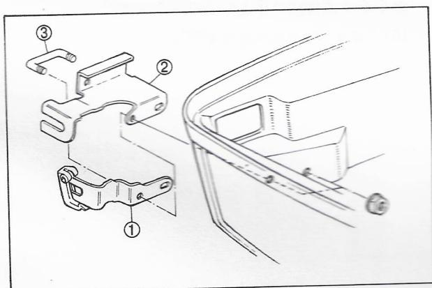
9. Below three parts should be assembled separately, as a sub assembly and installed to the bottom cowling.
