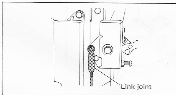
2. Remove the link joint first.
