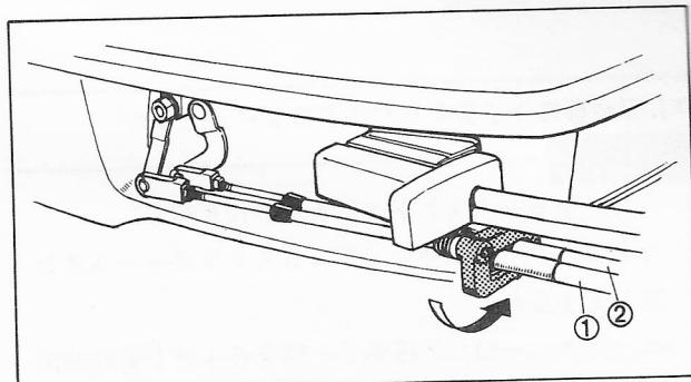
10. Connect the remote control cables to the remote control bracket.
